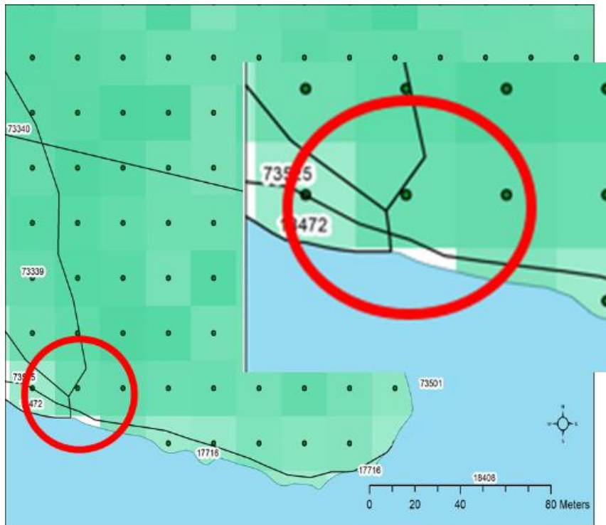
Figure 26 - Example of a raster pixel being bisected into 4 by polygon boundaries with only one polygon including the centroid value.
